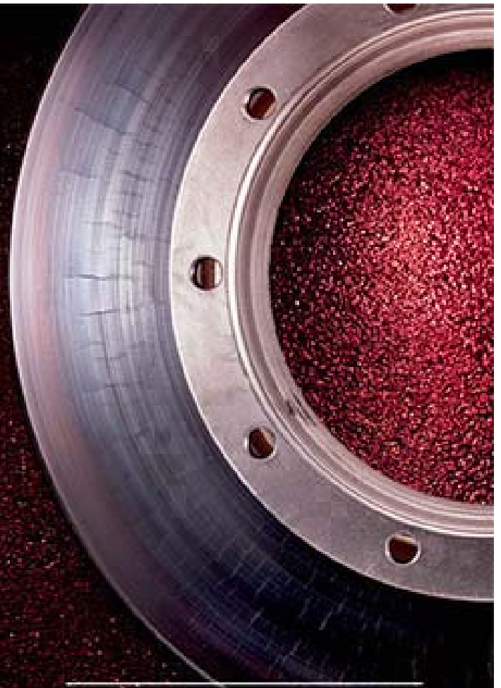
Original disks "Mercedes-Benz", after 150 of the 500 braking.
