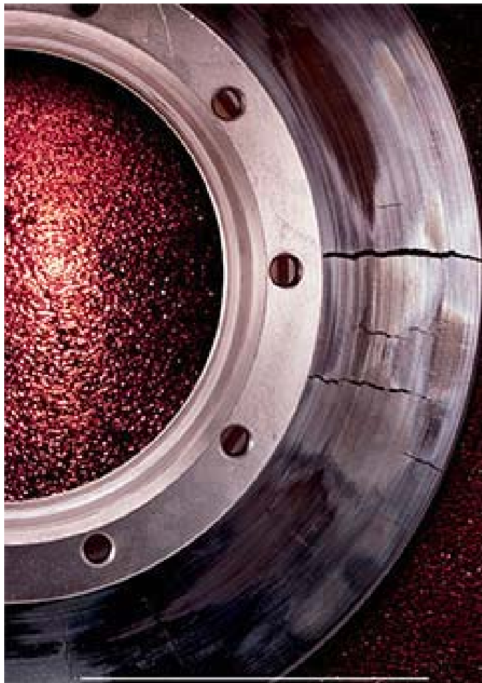
Disks of a competing manufacturer after 150 of 500 braking.
