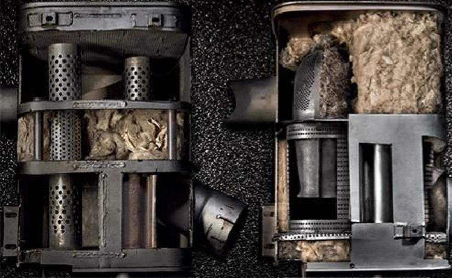
in the muffler of a competing manufacturer: little sound insulation material
